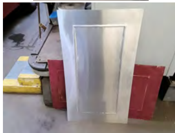
262's fire distorted aluminium panel, upper and its hand-made replacement with ornate radiused impression, lower.
