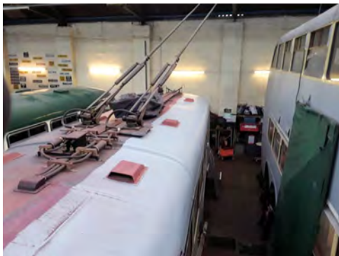
Lower right. Nearside roof of 243 painted with etch primer.
